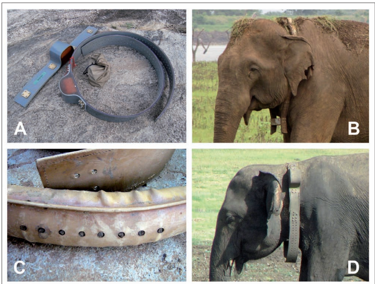
Figure 1. Elephant tracking collar configurations. (A) The two segments of a Telonics collar. (B) Single piece Vectronic collar with directly bolted counter weight at the bottom (AWT and Followit have a similar design). (C) Old Telonics collar belt filled with mud. (D) New Telonics collar slid to the side of the neck of a female.
