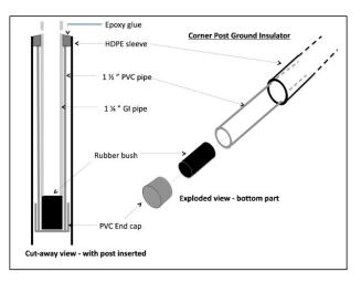
Figure 6. Detail of ground insulator for corner post.
