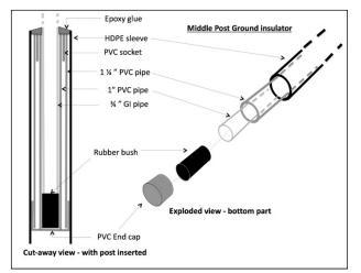
Figure 8. Ground insulator for middle post.
